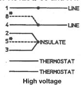
\*R5125Q-50 Blowers produced after September 1992 (Serial No. 0992) do not have motor leads 5 and 8.
