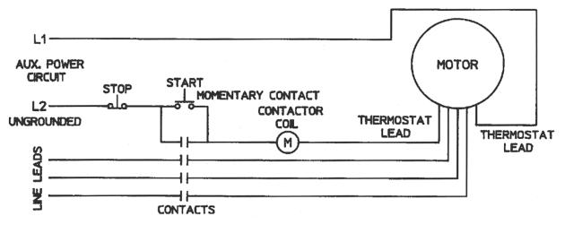
Thermostats to be connected in series with control as shown. Motor furnished with automatic thermostats rated A.C. 115-600V. 720VA circuit shown is for 3 phase motor. Single phase motor has two line leads in the above circuit.
