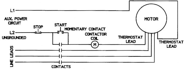
Thermostats to be connected in series with control as shown. Motor furnished with automatic thermostats rated A.C. 115-600V. 720VA circuit shown is for 3 phase motor. Single phase motor has two line leads in the above circuit.
