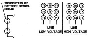
WARNING: This motor is thermally protected and will automatically restart when protector resets. Always disconnect power supply before servicing.
