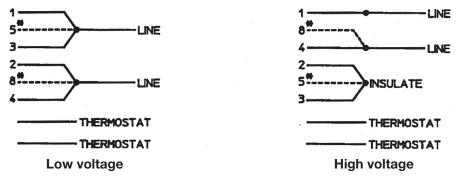
\*R5125Q-50 Blowers produced after September 1992 (Serial No. 0992) do not have motor leads 5 and 8.
