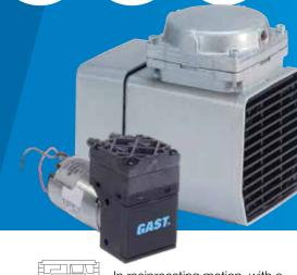
In reciprocating motion, with a short stroke, the diaphragm at the top of the connecting rod flexes up and down in a closed chamber, creating pressure or vacuum.
